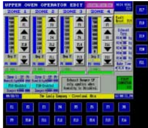
Typical PanelView control screen from a multi-zone oven application.
